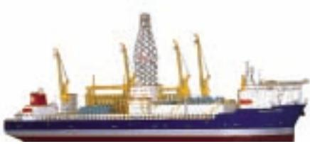
SAMSUNG HEAVY INDUSTRIES' DRILLSHIP CAN REACH DOWN TO CRUDE OIL AND NATURAL GAS 8,000 METERS BELOW THE SEA BOTTOM IN WATERS AS DEEP AS 3,000 METERS. STATIONARY OIL RIGS MUST BE ABANDONED AFTER A PARTICULAR FIELD PROVES FRUITLESS, BUT THE DRILLSHIP CAN SIMPLY BE MOVED TO ANOTHER FIELD, TO DRILL AGAIN ANOTHER DAY.
