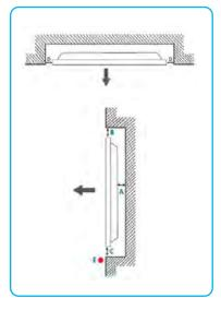
When installing the product on an indented wall, allow at least the space specified below between the product and wall for ventilation and ensure that the ambient temperature is kept below 35 °C.
